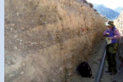
**Figure 6:** An example of possible seismic dislocations in soft rock in the trench wall, located near the temporal base for hydrocascade construction. The slanting wedges in the wall are presumably indications of seismogenic dislocations during historical earthquake events.
