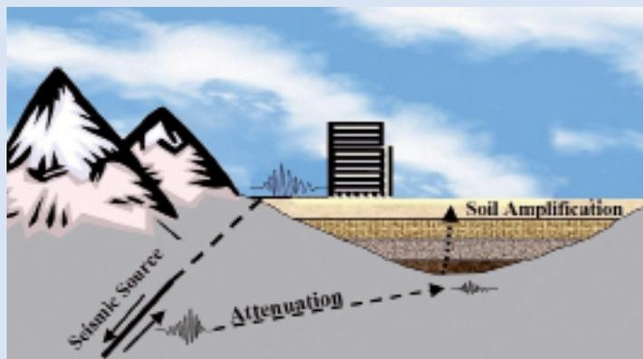
**Figure 3:** Hazard analysis is based on seismic source modelling, wave attenuation, and local ground amplification.
